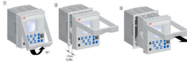
Figure-16 Removal of RER615 from its case
